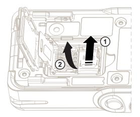
**5** Carefully insert the microSD card into the microSD card holder ensuring that the gold contact area is facing down.
