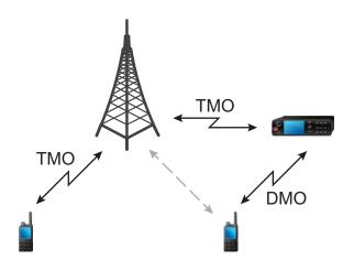
When the radio connects to a gateway, it plays a tone, displays the Gateway available message, and shows an appropriate icon. When the radio loses connection with the gateway, it plays a tone, displays the Gateway not available message, and the gateway icon is blinking.
