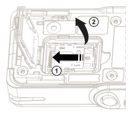
4 Slide the microSD card holder upward (as indicated by the UNLOCK arrow) and lift it up.
